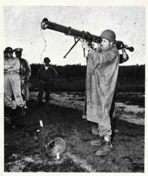
A GI in Korea came up with the idea of using rocket launcher to lay telephone wire across terrain that's under fire.
